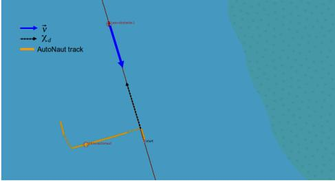
Fig. 12: Head-on with anti-grounding activated.
